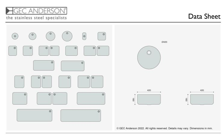
CG4.2 circular bowl: Ø420x180mm. Complete with Ø38mm waste and overflow fittings.
