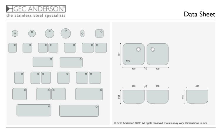
DG44 double bowls: 400x400x250mm. Complete with Ø38mm waste and overflow fittings.
