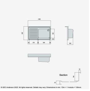
DR106 (G54) Decimetric® 1000x600mm - single bowl, single drainer - commercial grade stainless steel sinktop. 40mm lipped front and side edges and 100x20mm rear upstand. Bowl size: 500x400x250mm deep complete with Ø38mm outlet and overflow fittings. Sound deadened and plastic protected. (EN 1.4301 grade stainless steel). LH drainer.
