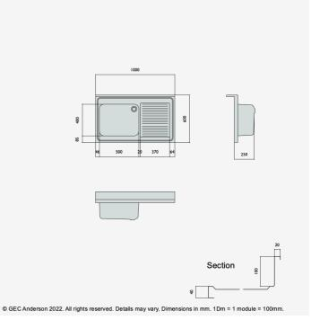
DR106 (G54) Decimetric® 1000x600mm - single bowl, single drainer - commercial grade stainless steel sinktop. 40mm lipped front and side edges and 100x20mm rear upstand. Bowl size: 500x400x250mm deep complete with Ø38mm outlet and overflow fittings. Sound deadened and plastic protected. (EN 1.4301 grade stainless steel). RH drainer.
