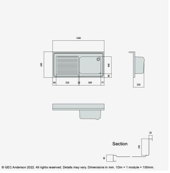
DR126 (G54) Decimetric® I200x600mm - single bowl, single drainer - commercial grade stainless steel sinktop. 40mm lipped front and side edges and I00x20mm rear upstand. Bowl size: 500x400x250mm deep complete with Ø38mm outlet and overflow fittings. Sound deadened and plastic protected. (EN I.4301 grade stainless steel). LH drainer.
