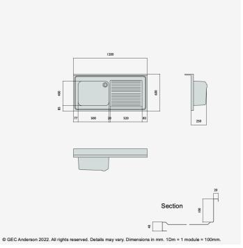
DR126 (G54) Decimetric® I200x600mm - single bowl, single drainer - commercial grade stainless steel sinktop. 40mm lipped front and side edges and I00x20mm rear upstand. Bowl size: 500x400x250mm deep complete with Ø38mm outlet and overflow fittings. Sound deadened and plastic protected. (EN I.4301 grade stainless steel). RH drainer.
