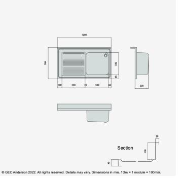
DR127 (G55) Decimetric® 1200x700mm - single bowl, single drainer - commercial grade stainless steel sinktop. 40mm lipped front and side edges and 100x20mm rear upstand. Bowl size: 500x500x300mm deep complete with Ø38mm outlet. Sound deadened and plastic protected. (EN 1.4301 grade stainless steel). LH drainer.
