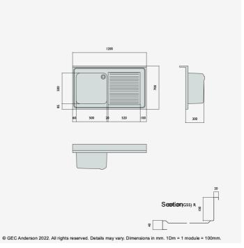
DR127 (G55) Decimetric® 1200x700mm - single bowl, single drainer - commercial grade stainless steel sinktop. 40mm lipped front and side edges and 100x20mm rear upstand. Bowl size: 500x500x300mm deep complete with Ø38mm outlet. Sound deadened and plastic protected. (EN 1.4301 grade stainless steel). RH drainer.
