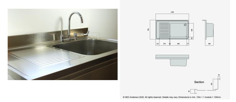
DR127 (G65) Decimetric® 1200x700mm - single bowl, single drainer - commercial grade stainless steel sinktop. 40mm lipped front and side edges and 100x20mm rear upstand. Bowl size: 600x500x320mm deep complete with Ø38mm outlet and overflow fittings. Sound deadened and plastic protected. (EN 1.4301 grade stainless steel). LH drainer.
