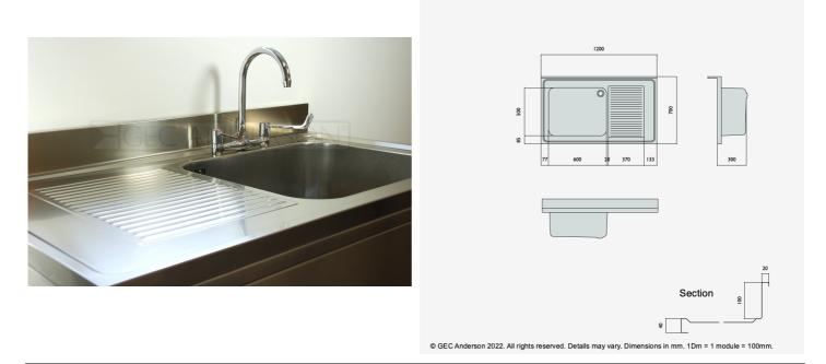
DR127 (G65) Decimetric® 1200x700mm - single bowl, single drainer - commercial grade stainless steel sinktop. 40mm lipped front and side edges and 100x20mm rear upstand. Bowl size: 600x500x320mm deep complete with Ø38mm outlet and overflow fittings. Sound deadened and plastic protected. (EN 1.4301 grade stainless steel). RH drainer.
