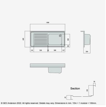
DR136 (G54) Decimetric® 1300x600mm - single bowl, single drainer - commercial grade stainless steel sinktop. 40mm lipped front and side edges and 100x20mm rear upstand. Bowl size: 500x400x250mm deep complete with Ø38mm outlet and overflow fittings. Sound deadened and plastic protected. (EN 1.4301 grade stainless steel). LH drainer.
