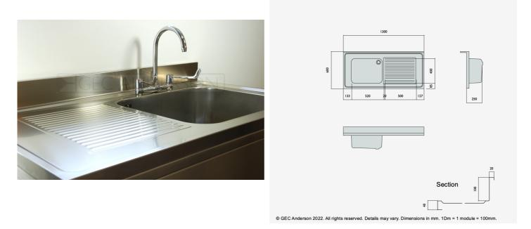
DR136 (G54) Decimetric® 1300x600mm - single bowl, single drainer - commercial grade stainless steel sinktop. 40mm lipped front and side edges and 100x20mm rear upstand. Bowl size: 500x400x250mm deep complete with Ø38mm outlet and overflow fittings. Sound deadened and plastic protected. (EN 1.4301 grade stainless steel). RH drainer.
