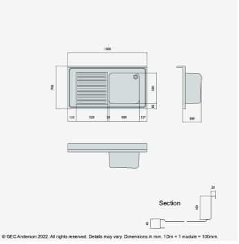
DR137 (G55) Decimetric® 1300x700mm - single bowl, single drainer - commercial grade stainless steel sinktop. 40mm lipped front and side edges and 100x20mm rear upstand. Bowl size: 500x500x300mm deep complete with Ø38mm outlet and overflow fittings. Sound deadened and plastic protected. (EN 1.4301 grade stainless steel). LH drainer.
