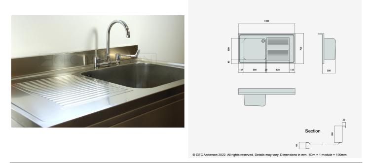
DR137 (G55) Decimetric® 1300x700mm - single bowl, single drainer - commercial grade stainless steel sinktop. 40mm lipped front and side edges and 100x20mm rear upstand. Bowl size: 500x500x300mm deep complete with Ø38mm outlet and overflow fittings. Sound deadened and plastic protected. (EN 1.4301 grade stainless steel). RH drainer.
