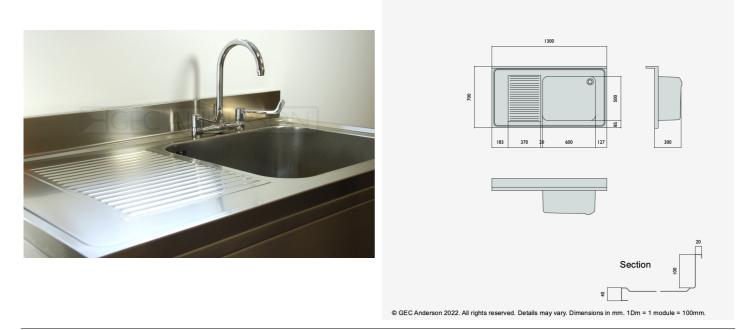
DR137 (G65) Decimetric® 1300x700mm - single bowl, single drainer - commercial grade stainless steel sinktop. 40mm lipped front and side edges and 100x20mm rear upstand. Bowl size: 600x500x320mm deep complete with Ø38mm outlet and overflow fittings. Sound deadened and plastic protected. (EN 1.4301 grade stainless steel). LH drainer.
