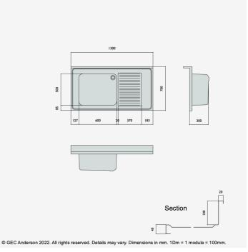
DR137 (G65) Decimetric® 1300x700mm - single bowl, single drainer - commercial grade stainless steel sinktop. 40mm lipped front and side edges and 100x20mm rear upstand. Bowl size: 600x500x320mm deep complete with Ø38mm outlet and overflow fittings. Sound deadened and plastic protected. (EN 1.4301 grade stainless steel). RH drainer.
