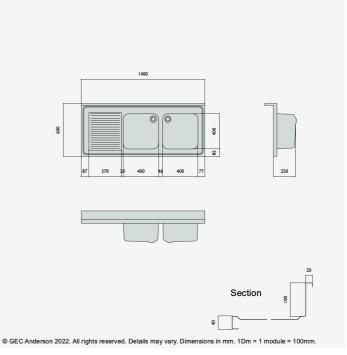
DR146 (DG44) Decimetric® I400x600mm - double bowl, single drainer - commercial grade stainless steel sinktop. 40mm lipped front and side edges and 100x20mm rear upstand. Bowl size: 400x400x250mm deep complete with Ø38mm outlet and overflow fittings. Sound deadened and plastic protected. (EN 1.4301 grade stainless steel). LH drainer.
