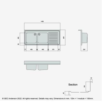
DR146 (DG44) Decimetric® I400x600mm - double bowl, single drainer - commercial grade stainless steel sinktop. 40mm lipped front and side edges and I00x20mm rear upstand. Bowl size: 400x400x250mm deep complete with Ø38mm outlet and overflow fittings. Sound deadened and plastic protected. (EN I.4301 grade stainless steel). RH drainer.
