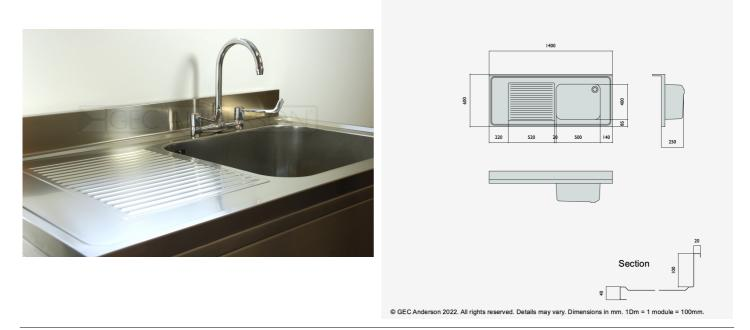
DR146 (G54) Decimetric® 1400x600mm - single bowl, single drainer - commercial grade stainless steel sinktop. 40mm lipped front and side edges and 100x20mm rear upstand. Bowl size: 500x400x250mm deep complete with Ø38mm outlet and overflow fittings. Sound deadened and plastic protected. (EN 1.4301 grade stainless steel). LH drainer.
