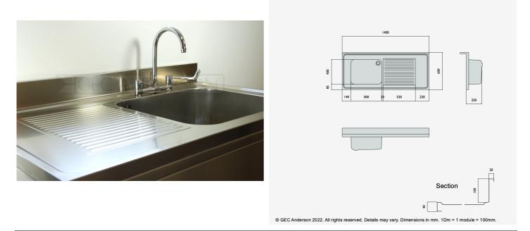
DR146 (G54) Decimetric® 1400x600mm - single bowl, single drainer - commercial grade stainless steel sinktop. 40mm lipped front and side edges and 100x20mm rear upstand. Bowl size: 500x400x250mm deep complete with Ø38mm outlet and overflow fittings. Sound deadened and plastic protected. (EN 1.4301 grade stainless steel). RH drainer.
