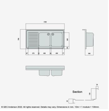
DR147 (DG45) Decimetric® 1400x700mm - double bowl, single drainer - commercial grade stainless steel sinktop. 40mm lipped front and side edges and 100x20mm rear upstand. Bowl size: 400x500x250mm deep complete with Ø38mm outlet and overflow fittings. Sound deadened and plastic protected. (EN 1.4301 grade stainless steel). LH drainer.
