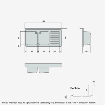
DR147 (DG45) Decimetric® 1400x700mm - double bowl, single drainer - commercial grade stainless steel sinktop. 40mm lipped front and side edges and 100x20mm rear upstand. Bowl size: 400x500x250mm deep complete with Ø38mm outlet and overflow fittings. Sound deadened and plastic protected. (EN 1.4301 grade stainless steel). RH drainer.
