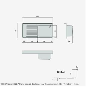
DR147 (G65) Decimetric® 1400x700mm - single bowl, single drainer - commercial grade stainless steel sinktop. 40mm lipped front and side edges and 100x20mm rear upstand. Bowl size: 600x500x320mm deep complete with Ø38mm outlet and overflow fittings. Sound deadened and plastic protected. (EN 1.4301 grade stainless steel). LH drainer.
