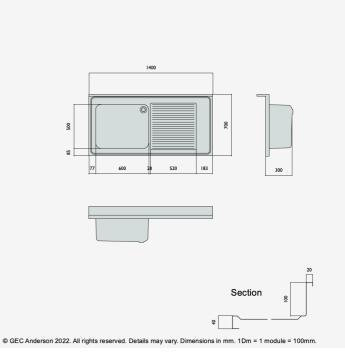
DR147 (G65) Decimetric® 1400x700mm - single bowl, single drainer - commercial grade stainless steel sinktop. 40mm lipped front and side edges and 100x20mm rear upstand. Bowl size: 600x500x320mm deep complete with Ø38mm outlet and overflow fittings. Sound deadened and plastic protected. (EN 1.4301 grade stainless steel). RH drainer.
