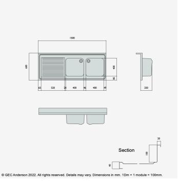
DR156 (DG44) Decimetric® 1500x600mm - double bowl, single drainer - commercial grade stainless steel sinktop. 40mm lipped front and side edges and 100x20mm rear upstand. Bowl size: 400x400x250mm deep complete with Ø38mm outlet and overflow fittings. Sound deadened and plastic protected. (EN 1.4301 grade stainless steel). LH drainer.
