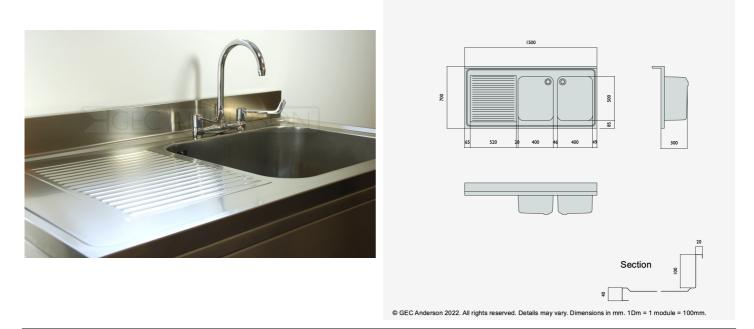
DR157 (DG45) Decimetric® 1500x700mm - double bowl, single drainer - commercial grade stainless steel sinktop. 40mm lipped front and side edges and 100x20mm rear upstand. Bowl size: 400x500x250mm deep complete with Ø38mm outlet and overflow fittings. Sound deadened and plastic protected. (EN 1.4301 grade stainless steel). LH drainer.
