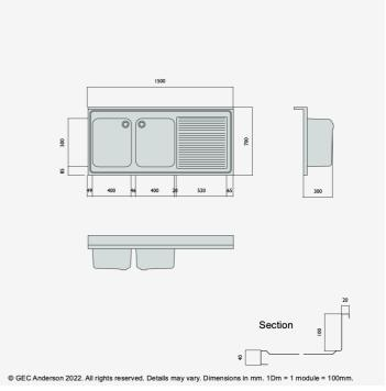
DR157 (DG45) Decimetric® 1500x700mm - double bowl, single drainer - commercial grade stainless steel sinktop. 40mm lipped front and side edges and 100x20mm rear upstand. Bowl size: 400x500x250mm deep complete with Ø38mm outlet and overflow fittings. Sound deadened and plastic protected. (EN 1.4301 grade stainless steel). RH drainer.
