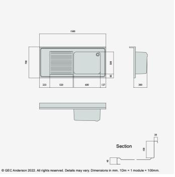
DR157 (G65) Decimetric® 1500x700mm - single bowl, single drainer - commercial grade stainless steel sinktop. 40mm lipped front and side edges and 100x20mm rear upstand. Bowl size: 600x500x320mm deep complete with Ø38mm outlet and overflow fittings. Sound deadened and plastic protected. (EN 1.4301 grade stainless steel). LH drainer.
