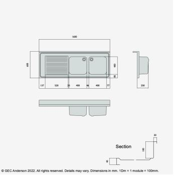
DR166 (DG44) Decimetric® 1600x600mm - double bowl, single drainer - commercial grade stainless steel sinktop. 40mm lipped front and side edges and 100x20mm rear upstand. Bowl size: 400x400x250mm deep complete with Ø38mm outlet and overflow fittings. Sound deadened and plastic protected. (EN 1.4301 grade stainless steel). LH drainer.
