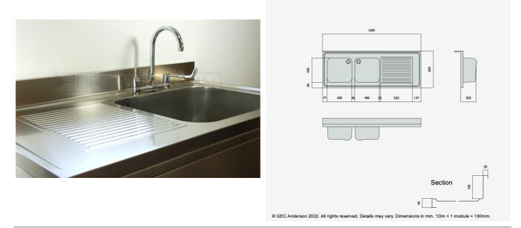
DR166 (DG44) Decimetric® 1600x600mm - double bowl, single drainer - commercial grade stainless steel sinktop. 40mm lipped front and side edges and 100x20mm rear upstand. Bowl size: 400x400x250mm deep complete with Ø38mm outlet and overflow fittings. Sound deadened and plastic protected. (EN 1.4301 grade stainless steel). RH drainer.
