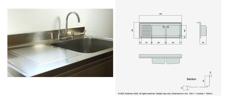
DR166 (DG54) Decimetric® 1600x600mm - double bowl, single drainer - commercial grade stainless steel sinktop. 40mm lipped front and side edges and 100x20mm rear upstand. Bowl size: 500x400x250mm deep complete with Ø38mm outlet and overflow fittings. Sound deadened and plastic protected. (EN 1.4301 grade stainless steel). LH drainer.
