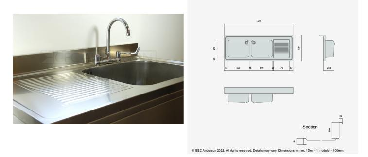
DR166 (DG54) Decimetric® 1600x600mm - double bowl, single drainer - commercial grade stainless steel sinktop. 40mm lipped front and side edges and 100x20mm rear upstand. Bowl size: 500x400x250mm deep complete with Ø38mm outlet and overflow fittings. Sound deadened and plastic protected. (EN 1.4301 grade stainless steel). RH drainer.
