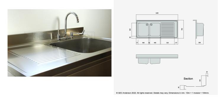
DR167 (DG45) Decimetric® 1600x700mm - double bowl, single drainer - commercial grade stainless steel sinktop. 40mm lipped front and side edges and 100x20mm rear upstand. Bowl size: 400x500x250mm deep complete with Ø38mm outlet and overflow fittings. Sound deadened and plastic protected. (EN 1.4301 grade stainless steel). RH drainer.
