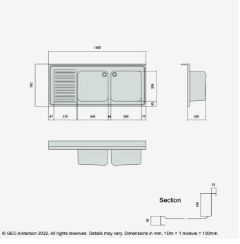
DR167 (DG55) Decimetric® 1600x700mm - double bowl, single drainer - commercial grade stainless steel sinktop. 40mm lipped front and side edges and 100x20mm rear upstand. Bowl size: 500x500x300mm deep complete with Ø38mm outlet and overflow fittings. Sound deadened and plastic protected. (EN 1.4301 grade stainless steel). LH drainer.
