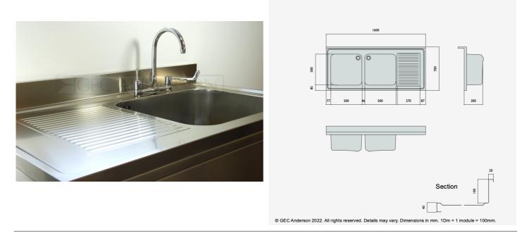
DR167 (DG55) Decimetric® 1600x700mm - double bowl, single drainer - commercial grade stainless steel sinktop. 40mm lipped front and side edges and 100x20mm rear upstand. Bowl size: 500x500x300mm deep complete with Ø38mm outlet and overflow fittings. Sound deadened and plastic protected. (EN 1.4301 grade stainless steel). RH drainer.
