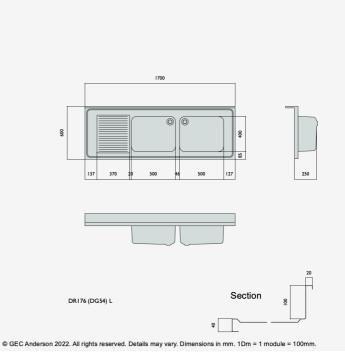
DR176 (DG54) Decimetric® 1700x600mm - double bowl, single drainer - commercial grade stainless steel sinktop. 40mm lipped front and side edges and 100x20mm rear upstand. Bowl size: 500x400x250mm deep complete with Ø38mm outlet and overflow fittings. Sound deadened and plastic protected. (EN 1.4301 grade stainless steel). LH drainer.
