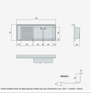
DR177 (DG45) Decimetric® 1700x700mm - double bowl, single drainer - commercial grade stainless steel sinktop. 40mm lipped front and side edges and 100x20mm rear upstand. Bowl size: 400x500x250mm deep complete with Ø38mm outlet and overflow fittings. Sound deadened and plastic protected. (EN 1.4301 grade stainless steel). LH drainer.
