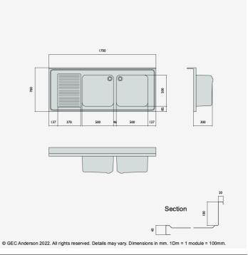
DR177 (DG55) Decimetric® 1700x700mm - double bowl, single drainer - commercial grade stainless steel sinktop. 40mm lipped front and side edges and 100x20mm rear upstand. Bowl size: 500x500x300mm deep complete with Ø38mm outlet and overflow fittings. Sound deadened and plastic protected. (EN 1.4301 grade stainless steel). LH Drainer.
