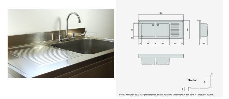
DR177 (DG55) Decimetric® 1700x700mm - double bowl, single drainer - commercial grade stainless steel sinktop. 40mm lipped front and side edges and 100x20mm rear upstand. Bowl size: 500x500x300mm deep complete with Ø38mm outlet and overflow fittings. Sound deadened and plastic protected. (EN 1.4301 grade stainless steel). RH drainer.
