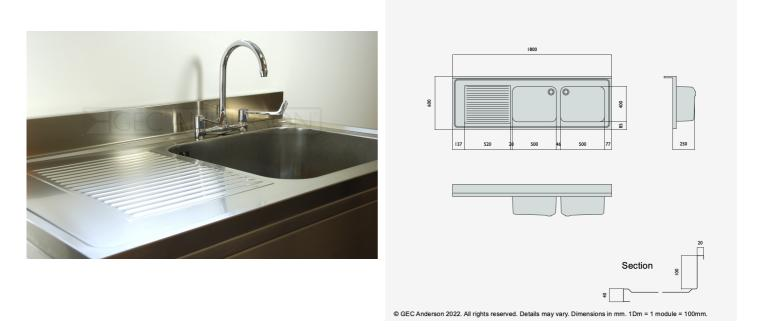
DR186 (DG54) Decimetric® 1800x600mm - double bowl, single drainer - commercial grade stainless steel sinktop. 40mm lipped front and side edges and 100x20mm rear upstand. Bowl size: 500x400x250mm deep complete with Ø38mm outlet and overflow fittings. Sound deadened and plastic protected. (EN 1.4301 grade stainless steel). LH drainer.
