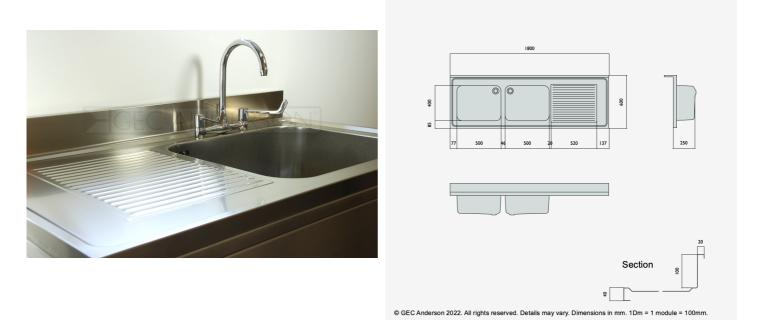
DR186 (DG54) Decimetric® 1800x600mm - double bowl, single drainer - commercial grade stainless steel sinktop. 40mm lipped front and side edges and 100x20mm rear upstand. Bowl size: 500x400x250mm deep complete with Ø38mm outlet and overflow fittings. Sound deadened and plastic protected. (EN 1.4301 grade stainless steel). RH drainer.
