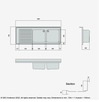
DR187 (DG55) Decimetric® 1800x700mm - double bowl, single drainer - commercial grade stainless steel sinktop. 40mm lipped front and side edges and 100x20mm rear upstand. Bowl size: 500x500x300mm deep complete with Ø38mm outlet and overflow fittings. Sound deadened and plastic protected. (EN 1.4301 grade stainless steel). LH drainer.
