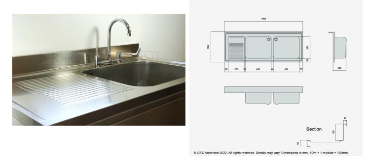
DR187 (DG65) Decimetric® 1800x700mm - double bowl, single drainer - commercial grade stainless steel sinktop. 40mm lipped front and side edges and 100x20mm rear upstand. Bowl size: 600x500x300mm deep complete with Ø38mm outlet and overflow fittings. Sound deadened and plastic protected. (EN 1.4301 grade stainless steel). LH drainer.
