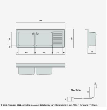
DR187 (DG65) Decimetric® 1800x700mm - double bowl, single drainer - commercial grade stainless steel sinktop. 40mm lipped front and side edges and 100x20mm rear upstand. Bowl size: 600x500x300mm deep complete with Ø38mm outlet and overflow fittings. Sound deadened and plastic protected. (EN 1.4301 grade stainless steel). RH drainer.
