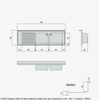
DR196 (DG54) Decimetric® 1900x600mm - double bowl, single drainer - commercial grade stainless steel sinktop. 40mm lipped front and side edges and 100x20mm rear upstand. Bowl size: 500x400x250mm deep complete with Ø38mm outlet and overflow fittings. Sound deadened and plastic protected. (EN 1.4301 grade stainless steel). LH drainer.
