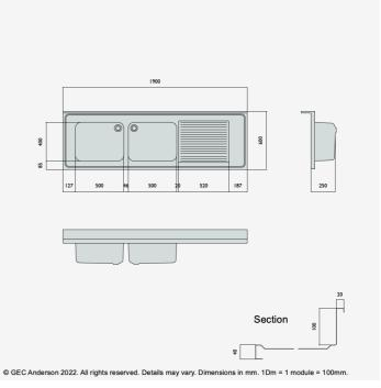
DR196 (DG54) Decimetric® 1900x600mm - double bowl, single drainer - commercial grade stainless steel sinktop. 40mm lipped front and side edges and 100x20mm rear upstand. Bowl size: 500x400x250mm deep complete with Ø38mm outlet and overflow fittings. Sound deadened and plastic protected. (EN 1.4301 grade stainless steel). RH drainer.
