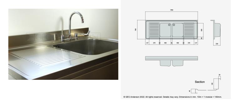
DR197 (DG45) Decimetric® 1900x700mm - double bowl, double drainer - commercial grade stainless steel sinktop. 40mm lipped front and side edges and 100x20mm rear upstand. Bowl size: 400x500x250mm deep complete with Ø38mm outlet and overflow fittings. Sound deadened and plastic protected. (EN 1.4301 grade stainless steel).
