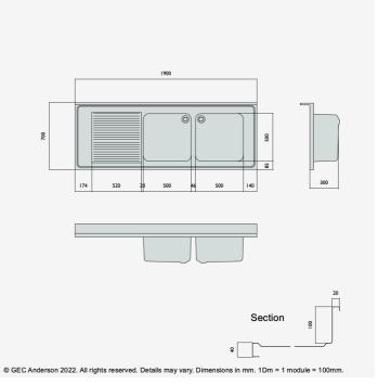
DR197 (DG55) Decimetric® 1900x700mm - double bowl, single drainer - commercial grade stainless steel sinktop. 40mm lipped front and side edges and 100x20mm rear upstand. Bowl size: 500x500x300mm deep complete with Ø38mm outlet and overflow fittings. Sound deadened and plastic protected. (EN 1.4301 grade stainless steel). LH drainer.
