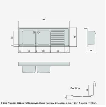
DR197 (DG55) Decimetric® 1900x700mm - double bowl, single drainer - commercial grade stainless steel sinktop. 40mm lipped front and side edges and 100x20mm rear upstand. Bowl size: 500x500x300mm deep complete with Ø38mm outlet and overflow fittings. Sound deadened and plastic protected. (EN 1.4301 grade stainless steel). RH drainer.
