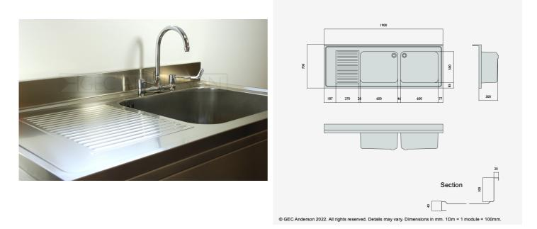
DR197 (DG65) Decimetric® 1900x700mm - double bowl, single drainer - commercial grade stainless steel sinktop. 40mm lipped front and side edges and 100x20mm rear upstand. Bowl size: 600x500x320mm deep complete with Ø38mm outlet and overflow fittings. Sound deadened and plastic protected. (EN 1.4301 grade stainless steel). LH drainer.
